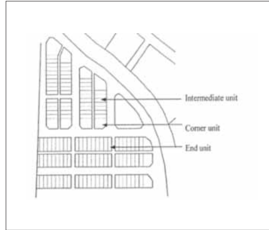
Figure 3: A Typical Layout of Terrace Housing in Urban Area, Malaysia. (Source: Authors).
