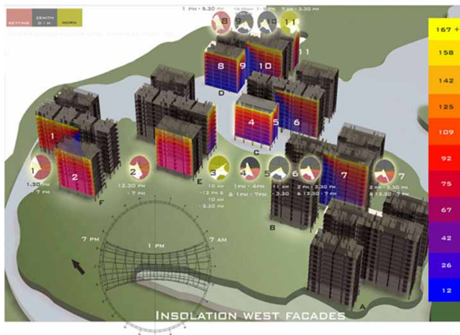
Figure 2: Insolation Study to Identify the Total Incident Radiation in \text{W/m}^2
